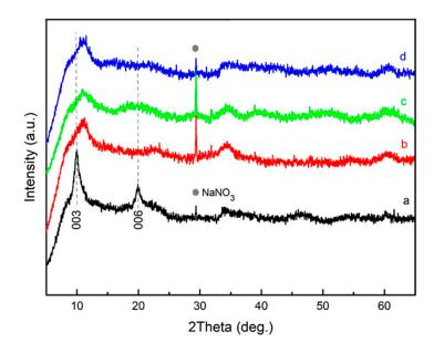
**Figure 1.** X-ray diffraction (XRD) patterns of the  $Co_2Al$ – $NO_3$  layered double hydroxides (LDHs) synthesized using the conventional co-precipitation method (**a**) and by means of the ultrasonic treatment of the stoichiometric mixture of the respective metal nitrates at 1.5 kW for 3 min (**b**), 5 min (**c**), and 10 min (**d**) followed by 4-h thermal treatment in a water bath. The strongest peak of the residual sodium nitrate (from the parent solution) is indicated.
