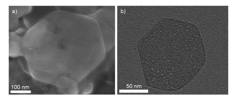
**Figure 7.** Electron microscope images of typical crystallites of Co<sub>2</sub>Al–NO<sub>3</sub> LDH were taken in scanning mode (**a**) and in scanning transmission mode (**b**).
