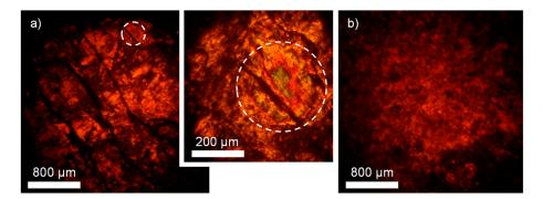
**Figure 5.** Images of the  $Co_2Al-CO_3$  samples in a polarized microscope: the pressed compact of the LDH powder precipitated in an external magnetic field and then dried without mixing (**a**) and the pressed compact of the LDH powder dried after centrifugation (**b**). Inset shows the magnified image of the zone with the iridescent colors.
