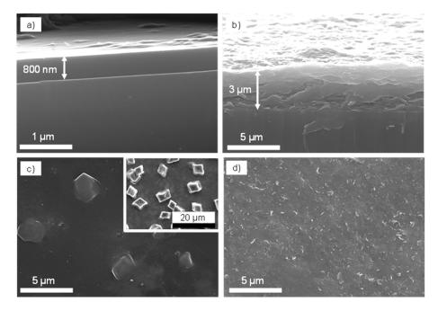
**Figure 8.** SEM images of layers of the  $Co_2Al-NO_3$  LDH crystallites deposited on glass substrates with (**a**,**c**) and without (**b**,**d**) application of an external magnetic field; cross section views (**a**,**b**) and top views (**c**,**d**). Inset shows the regular-shape particles of  $Co_2Al-NO_3$  formed on the surface of dense LDH film.
