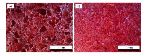
**Figure 4.** Images of the  $Co_2Al-NO_3$  samples in nonpolarized light: the pressed compact of the LDH powder precipitated in an external magnetic field and then dried without mixing (**a**) and the pressed compact of the LDH powder dried after centrifugation (**b**).
