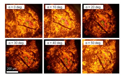
**Figure 6.** Images of the Co<sub>2</sub>Al–CO<sub>3</sub> LDH compact (the same sample that shown in Figure 5a) in crossed polarizers. The turning angles of the sample in the microscope stage ( $\alpha$ ) are indicated.
