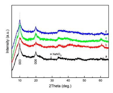
**Figure 2.** XRD patterns of the  $Co_2Al-NO_3$  LDHs synthesized using the conventional co-precipitation method and then either kept in a water bath at about 100 °C for 4 h (a) or sonicated at 1.5 kW for 2 min (b), 5 min (c), and 10 min (d).
