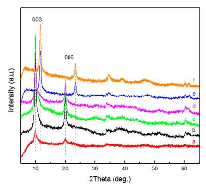
**Figure 3.** XRD patterns of the Co<sub>2</sub>Al–NO<sub>3</sub> LDH prepared using the conventional co-precipitation method before (**a**), after the NO<sub>3</sub><sup>-</sup>  $\rightarrow$  CO<sub>3</sub><sup>2-</sup> anion-exchange reaction at room temperature either without sonication for 7 min (**b**), 60 min (**c**), 24 h (**d**) and 7 days (**f**) or under a 1.5 kW sonication for 7 min (**e**).
