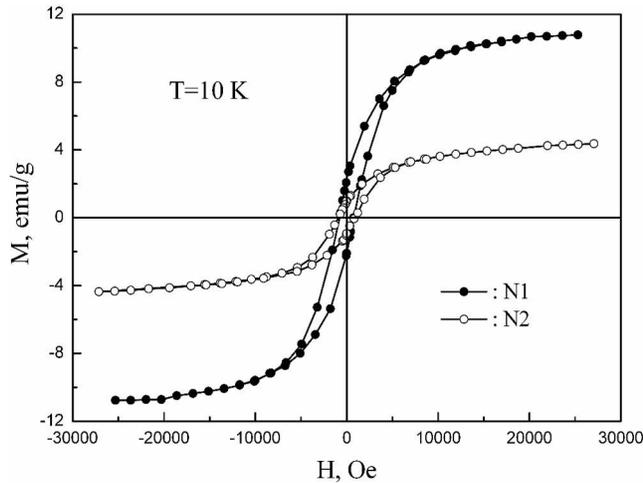
**Figure 3.** Magnetization curves at  $T = 10$  K for samples MWCNTs (ferrocene, cyclohexane, N1) and N-MWCNTs (ferrocene, acetonitril, N2).
