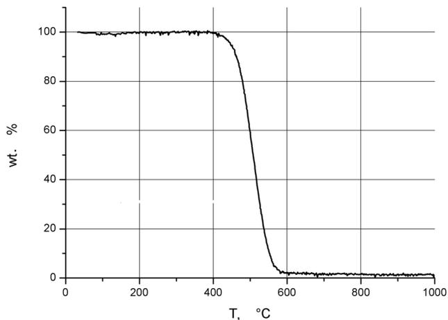
**Figure 1.** TG measurements of N-MWCNTs (heating rate 1 K/min in air).
