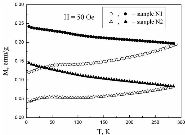
**Figure 2.** Temperature dependence of magnetization in  $H = 50$  Oe for samples MWCNT (ferrocene, cyclohexane, N1) and N-MWCNT (ferrocene, acetonitril, N2). Open and full symbols correspond to ZFC and FC regimes, respectively.
