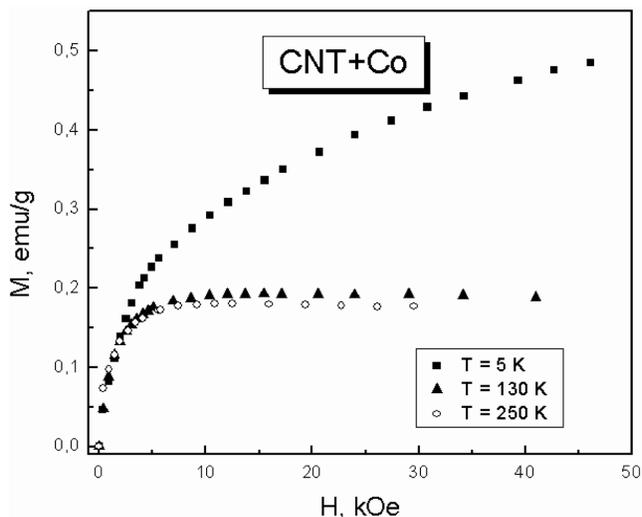
**Fig. 4.** Magnetization of MWCNT + Co at temperatures 5, 130, and 250 K.
