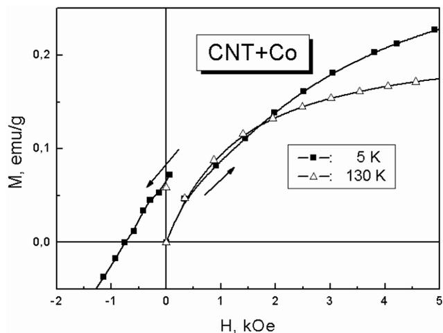
**Fig. 5.** Hysteresis effects in magnetization of MWCNT+Co at temperatures 5 and 130 K.
