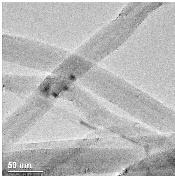
**Fig. 2.** SEM and HRTEM pictures of the MWCNT with Cobalt. Dark spots denote metal nanoparticles (Pictures taken with: SEM FEI XL30 LaB<sub>6</sub>; HRTEM Philips TECNAI 20 S-TWIN).
