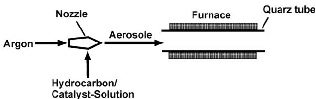
**Fig. 1.** Principle scheme of a spray pyrolysis reactor for the production of CNT
